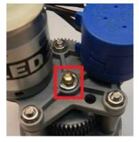
19. Secure the two screws 3x8 (8) to the superior support (17)
