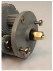
20. Mount the drum (18) on the mast (14) locking it with the washer (10) and the screw  $3\times8$  (8)
