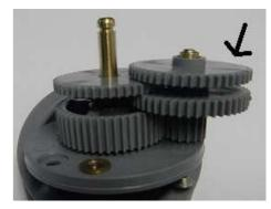
12. On the lower support of the winch (9) mount the motor (20) with the two selftapping screws (5) and the drive pinion (15)
