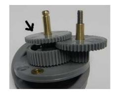
11. On the distance tube (11) assemble the gear (3)
